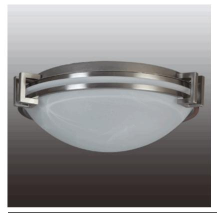
12.25" Brushed Nickel Ceiling fixture, 4" Deep, two GU24 sockets, direct wired, with White Swirl Glass Diffuser. Recommend two 800 lumen LED bulbs with GU24 base.
